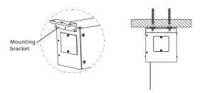
Leave at least 1000mm spare distance on the left edge referring to ceiling hanging/ceiling mounted installation. Fix the left and right mounting brackets with screws onto wall
